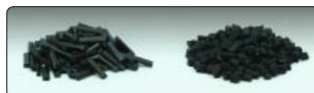
C4LF™ raw material (at left) compared to standard carbon fiber material, showing the longer fiber length.
